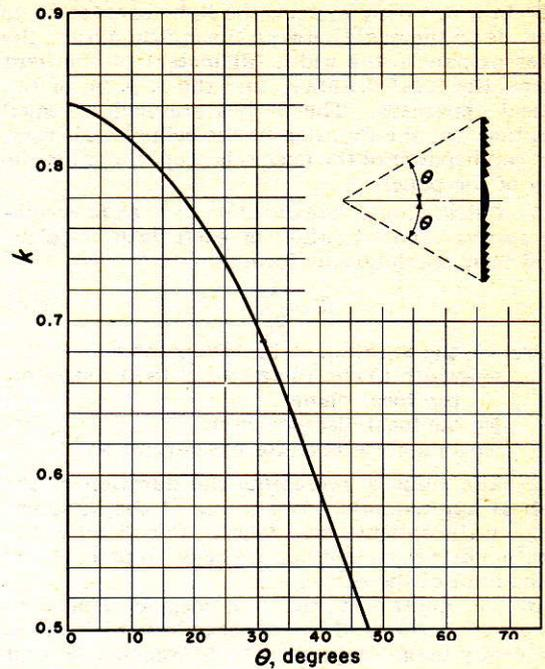
FIGURE 23-16.—Graph of a pencil beam symmetrical dioptric.
