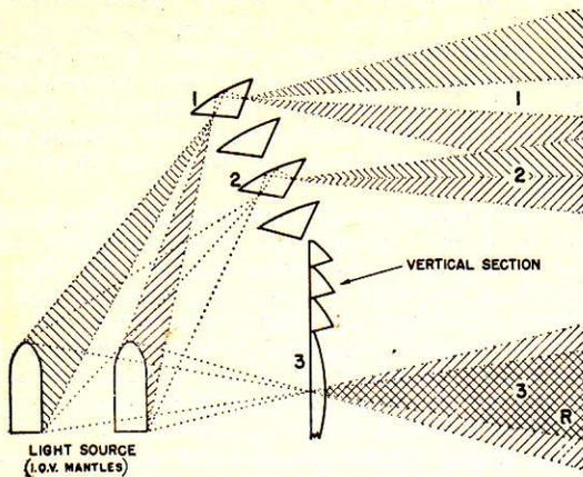
FIGURE 23-18.—Multiple light source in fixed lens.
