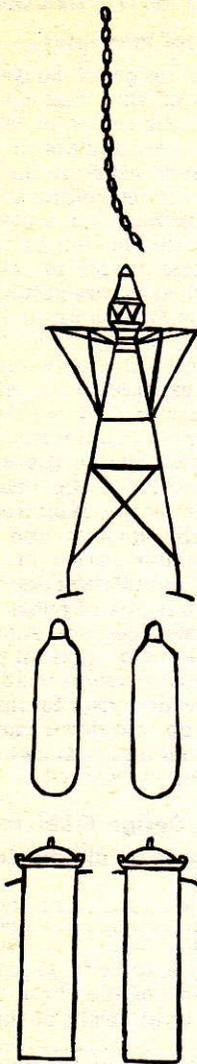
FIGURE 23-25.—Weights which a buoy must support.
