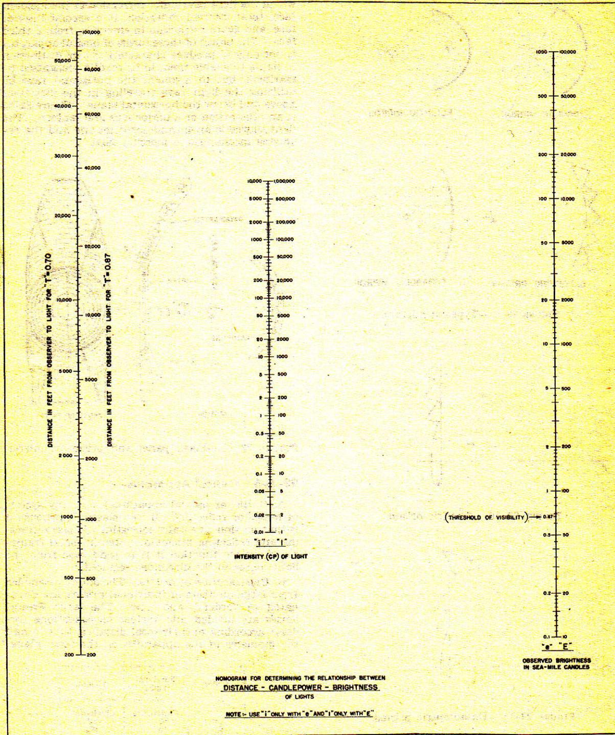
FIGURE 23-8.—Nomogram for determining the relationship between Distance — Candlepower — Brightness.
