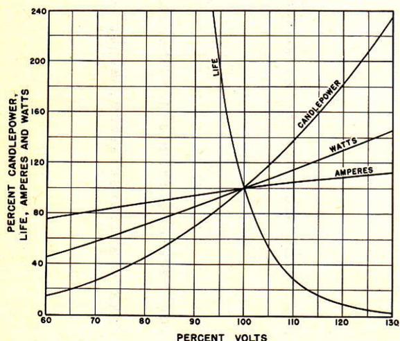
FIGURE 23-24.—Effect of voltage change on characteristics of small lamps.
