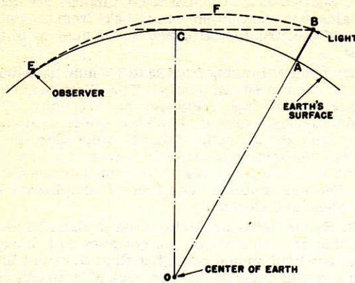
FIGURE 23-5.—Effect of refraction on geographic range.
