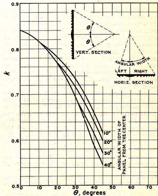
FIGURE 23-17.—Graph of a pencil beam asymmetrical dioptric.
