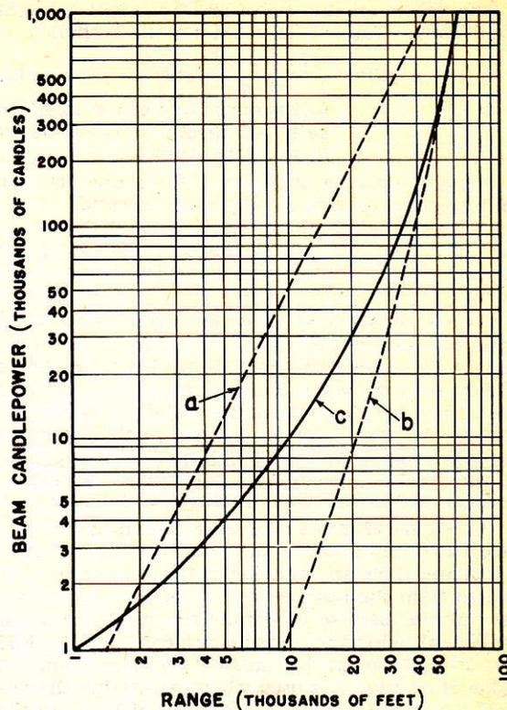
FIGURE 23-7.—Daylight visibility of range lights.
