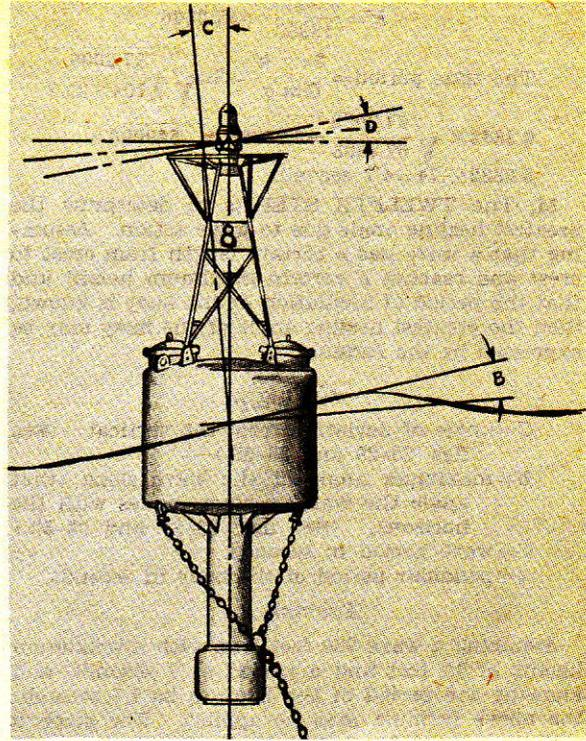
FIGURE 23-30.—An 8 x 26 buoy in a seaway.
