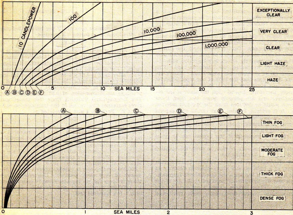
FIGURE 23-4.—Luminous range for different atmospheric conditions.
