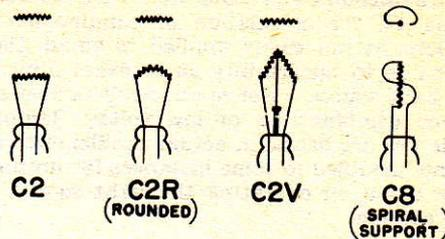
FIGURE 23-21.—Low voltage filament types.
