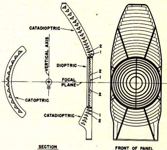
FIGURE 23-12.—Flash panel and prismatic mirror.
