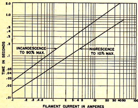
FIGURE 23-22.—Heating and cooling time of gas-filled lamps.
