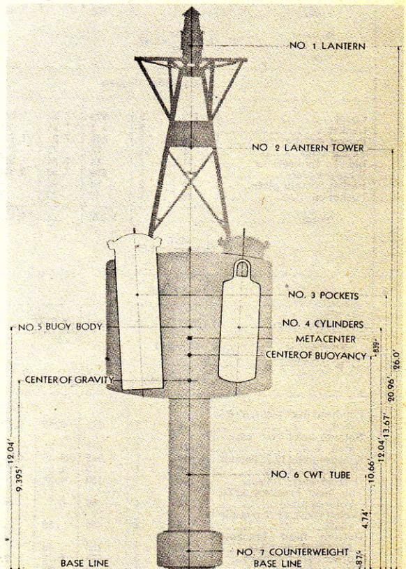
FIGURE 23-28.—An 8x26 buoy.
