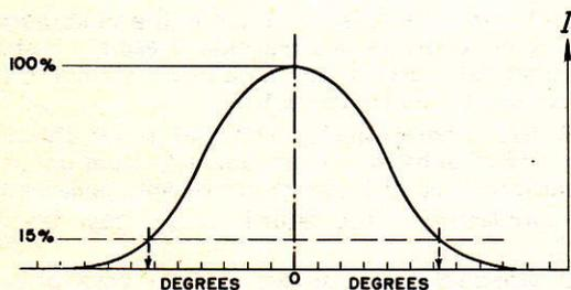
FIGURE 23-2.—Typical candlepower distribution.
