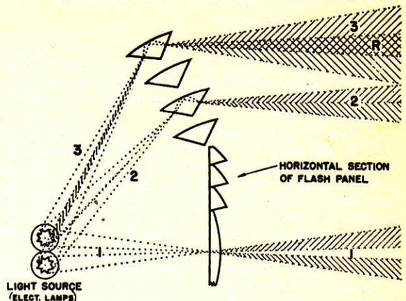
FIGURE 23-19.—Effect of multiple light source on candlepower and flash length in revolving apparatus.
