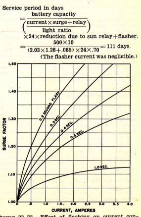
FIGURE 23-23.—Effect of flashing on current consumption of small lamps.
