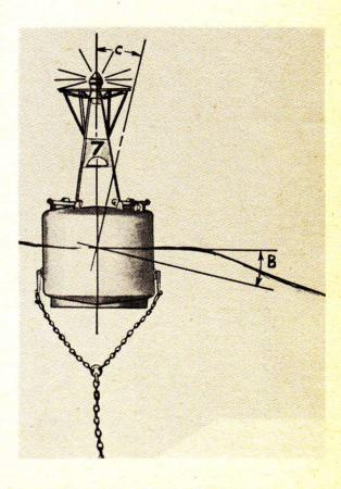
FIGURE 23-29.--- A 7 FE buoy in a seaway.
