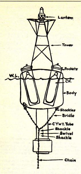
FIGURE 23-27.—Sketch of a buoy fulfilling requirements of buoy problem.
