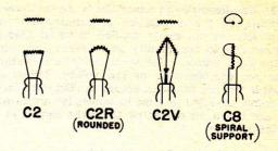
FIGURE 23-21.--Low voltage filament types.
