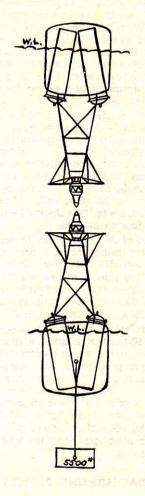
FIGURE 23-25.—Weights which a buoy must support.
