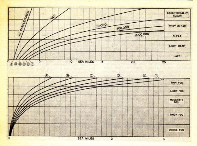
FIGURE 23-4.—Luminous range for different atmospheric conditions.
