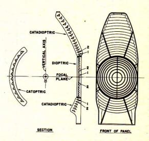
FIGURE 23-12.-Flash panel and prismatic mirror.
