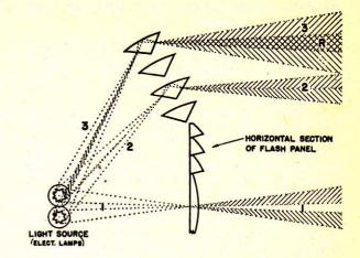
FIGURE 23–19.—Effect of multiple light source on candlepower and flash length in revolving apparatus.
