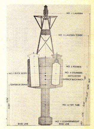
FIGURE 23-28.-An 8×26 buoy.
