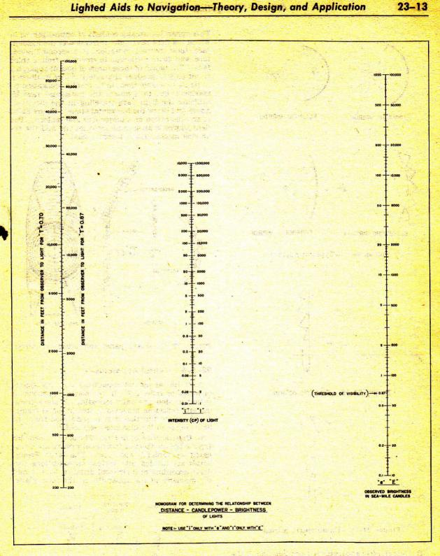
FIGURE 23-8.-Nomogram for determining the relationship between Distance - Candlepower -Brightness.
