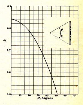
FIGURE 23-14.—Graph of a fan beam dioptric.
